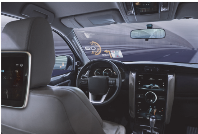
Figure 2: holistic HMIs enable to dynamically use content across multiple displays
