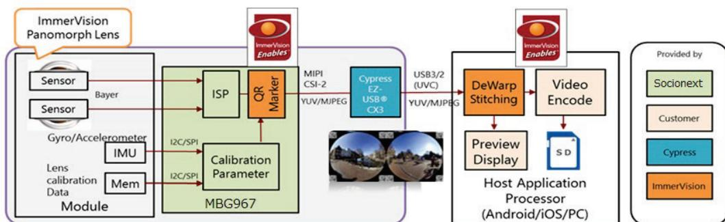
Fig. 3: USB Camera Configuration with MBG967
